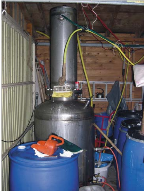
Steel reaction vessel of 120 litres capacity used in the clandestine production of amphetamine in a facility dismantled in Loosdrecht, the Netherlands (2003). Source: KLPD, the Netherlands.
