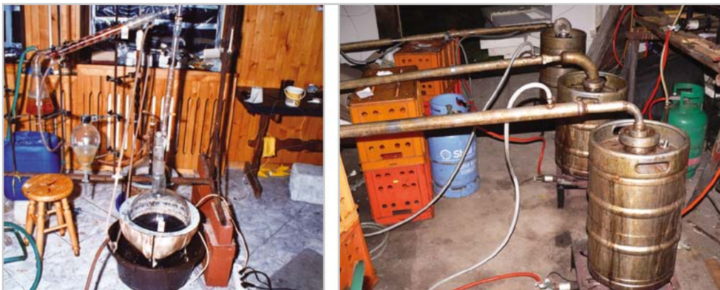
Reaction vessels of 20 litres (left) and 50 litres (right) capacity used in the distillation process in dismantled clandestine amphetamine production facilities at Kobytka (2002) and Puchaty (2008), respectively, both in Poland. Source: Central Bureau of Investigation, National Police Headquarters, Warsaw.
