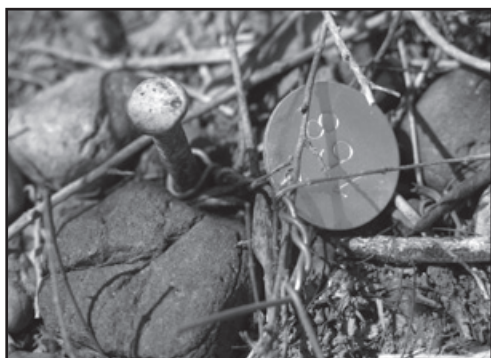
Aluminum tag secured with nine-inch nail.
